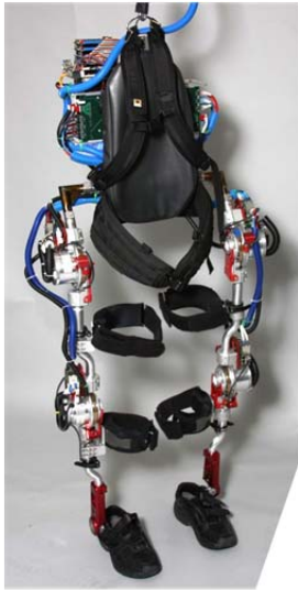
Figure 1: IHMC Mina, a robotic orthosis for assisting mobility. Mina has four actuated degrees of freedom. To date it has enabled individuals with paraplegia to walk on flat ground up to 0.2 m/s.
